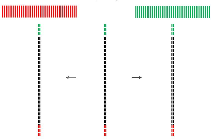
The PCR product is stripped of unused nucleotides and primers, divided in half, and each half is sequenced using a single primer.
