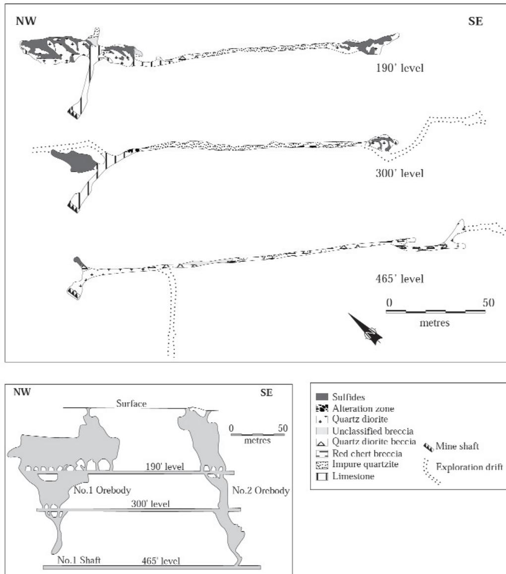
FIG. 13. Geologic cross section of the Milnet mine. Upper illustration shows simplified plan geology taken from mine plans. Lower illustration shows the shapes of the orebodies in vertical cross sectional view. Modified after Meyn (1970).
