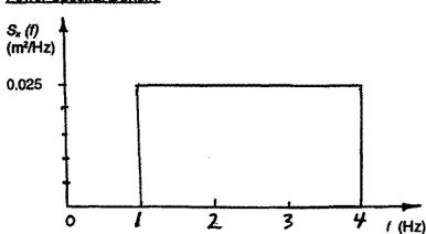
(8) a) Estimate the maximum (largest) value of x(t) expected within a time interval of T = 1 hour. (Hint; use the spectrum to determine  $\sigma_x$  and the cycling rate).
