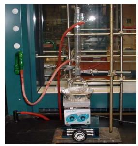
Equip the flask for simple distillation with a heating mantle. Distil the mixture rapidly into an ice-cooled flask until the head temperature reaches 120°C. Codistillation of 1-bromobutane and water occurs, and the increased boiling point is due to the codistillation of sulfuric acid and hydrobromic acid with water.
