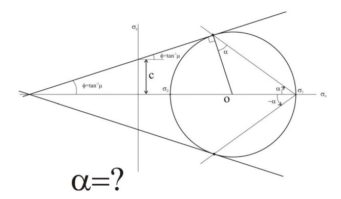
Orientation of shear fractures with respect to the principal stresses.
