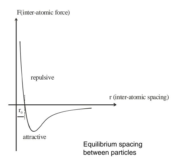
Schematic diagram showing the inter-atomic force as a function of inter-atomic spacing.
