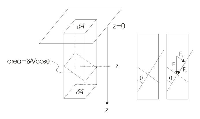
The total force is still the same, but now the area of action is increased. In addition, the stress has both a component of pure compression and a component of shear.
