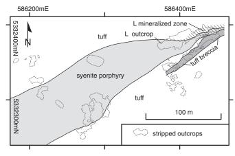
FIG. 13. Location map of stripped outcrops west of Upper Canada shaft 2, showing the distribution of major rock types. (Outcrop outlines modified from D.J. Toogood, unpub. report for Queenston Mining Inc., 1989, 57 p.). Coordinates are UTM zone 17 NAD 83.
