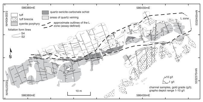
FIG. 14. Geologic map of the L stripped outcrop (outcrop outlines and gold grade graphs are from D.J. Toogood, unpub. report for Queenston Mining Inc., 1989, 57 p.). Graphs depict gold grades from 1 to greater than 10 g/t (i.e., gold grades >10 g/t are not differentiated). Coordinates are UTM zone 17 NAD 83.
