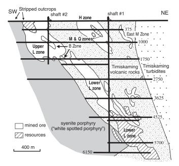
FIG. 12. Upper Canada mine, vertical longitudinal section, looking northwest (modified from Stevenson et al., 1995, and Queenston Mining Inc., Annual Report, 1996, 14 p.).
