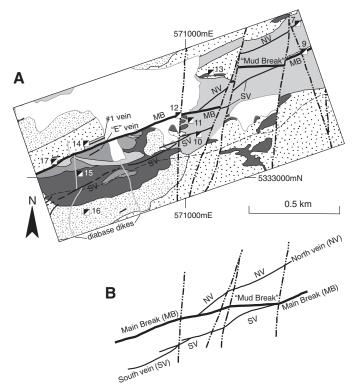
FIG. 4. A. Geology of the central part of the Kirkland Lake gold deposit (parts of Teck Hughes, Lake Shore, and Wright-Hargreaves properties), showing location of Teck Hughes 1 and "E" veins, and the "Mud Break." Same legend as Figure. 3. Based on Todd (1928), Thomson (1945), and Ispolatov (2005). B. Ore-hosting structures reconstructed "without" postore fault displacement. Coordinates are UTM zone 17 NAD 83.
