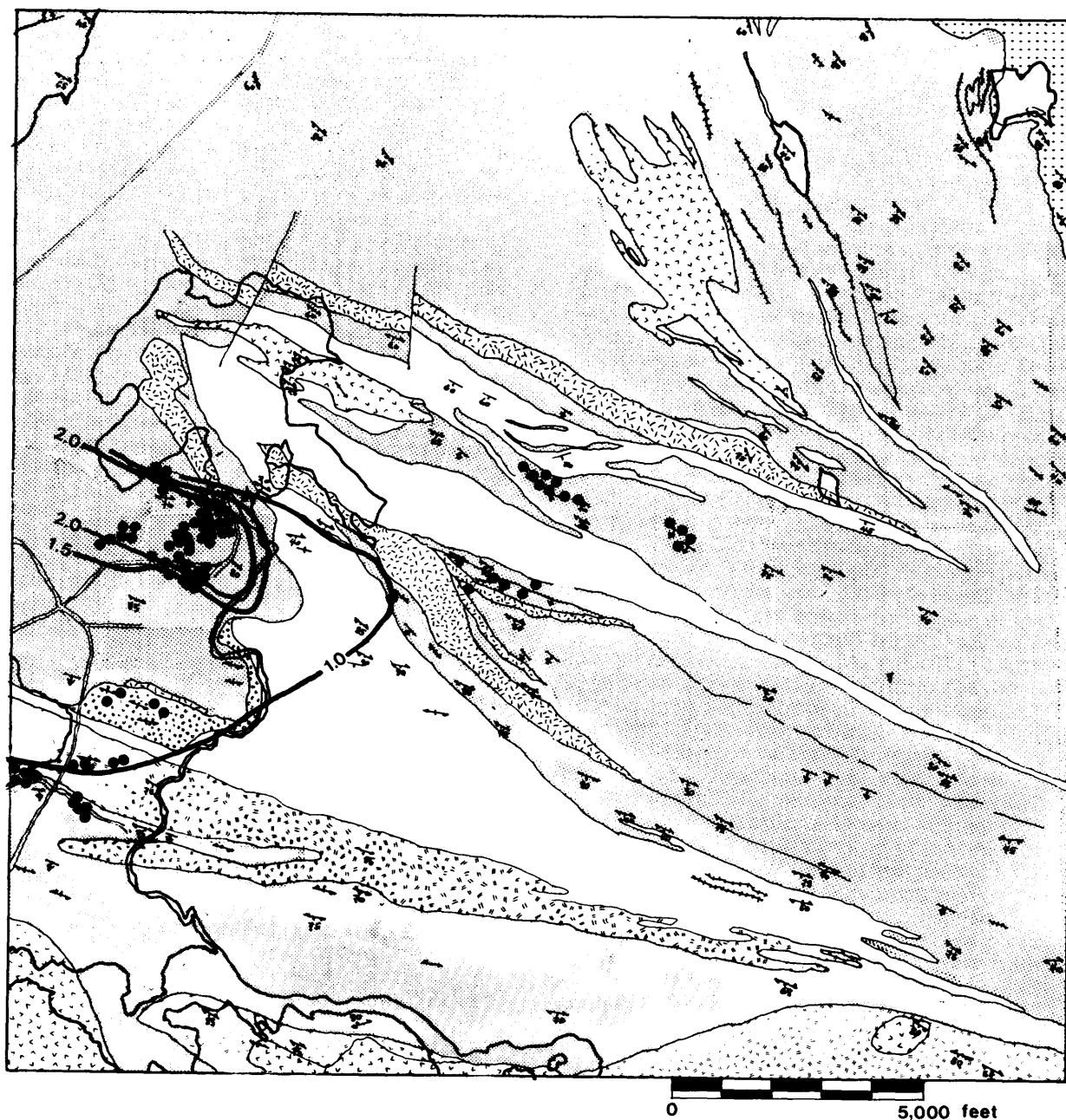
Figure 8-10—Contoured Peraluminosity Index (Mole percent Al_2O_3/(Na_2O + K_2O + CaO) ); (Spitz 1973) plot of analyzed samples (filled circles) in Balmer Township.
