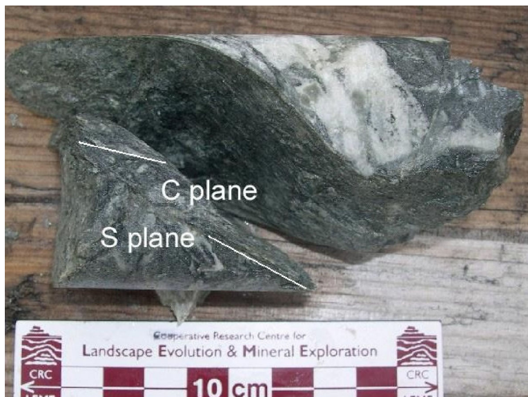
Photo 14. C-S fabric in intensely deformed Hersey Lake komatiites within the Porcupine–Destor deformation zone. These structures indicate dip-slip movement on a south-dipping zone of high strain. Drill core, hole 18986, from near Pamour mine (Porcupine Joint Venture).
