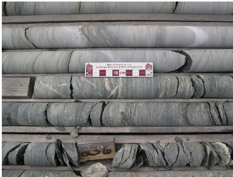
Photo 6. There is an angular discordance in foliation across the Timiskaming–Tisdale contact in places within the Porcupine–Destor deformation zone. The sediments are much less deformed than the volcanics. Drill hole 18964, south of Pamour pit, Whitney Township (Porcupine Joint Venture).
