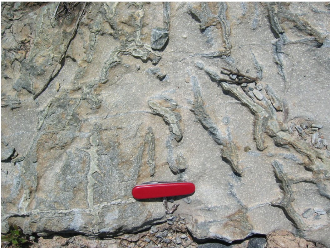
Photo 15. Epidote - chlorite - feldspar \pm carbonate stringers in intermediate metavolcanic rocks are interpreted to represent metamorphosed hydrothermal alteration associated with base metal mineralization in northwest Burt Township. Knife is 8 cm long. Outcrop located at 544718E, 5326582N, NAD 83, zone 17.
