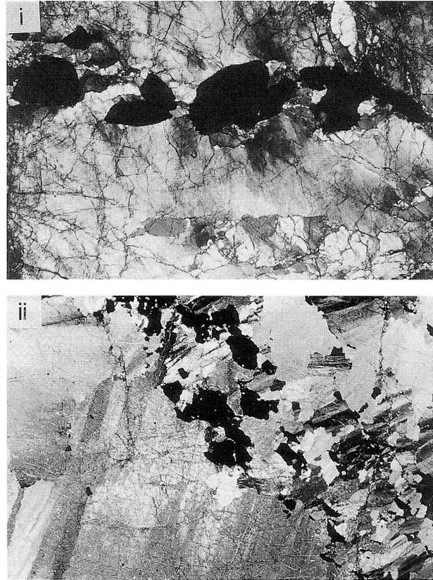
Fig. 4 Silicate rocks adjacent to a chromitite. i) Stringer of euhedral chromite (black) in a larger olivine grain (under polarized light, 3mm across); and ii) Euhedral chromite forming a chain of grains in a dunite vein (under polarized light, 6mm across).
