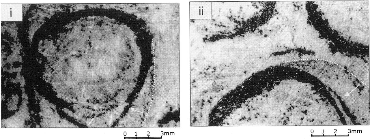
Fig. 3 i) and ii) Orbicular (ring-shaped) chromitites set in dunite with disseminated chromite (black). Thin chromite rings form shells at an early stage of the development of nodular texture. Note that the shifting of the shells can be traced as the shells are condensing. Dotted lines mark the previous shells of chromite, and arrows show the direction of collapse.
