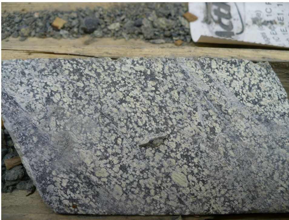
Figure 3.15. Up to 20 modal % very fine interstitial chromite hosted in light green fine grained serpentinized olivine, forming olivine-chromite heteradcumulate. Sample is from 59 m in DDH BT-08-10.
