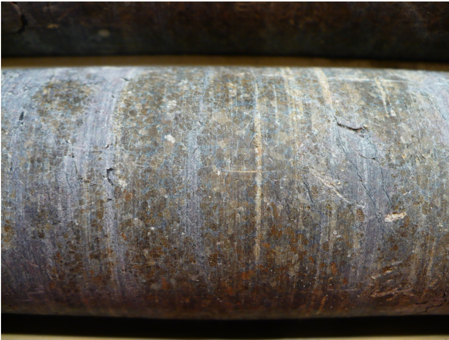
Figure 3.53. Primary bronzite in pyroxenite distinguished by their bronze colours and cleavage. Sample is from 34 m in DDH FW-12-108. Diameter of core is 46.7 mm.
