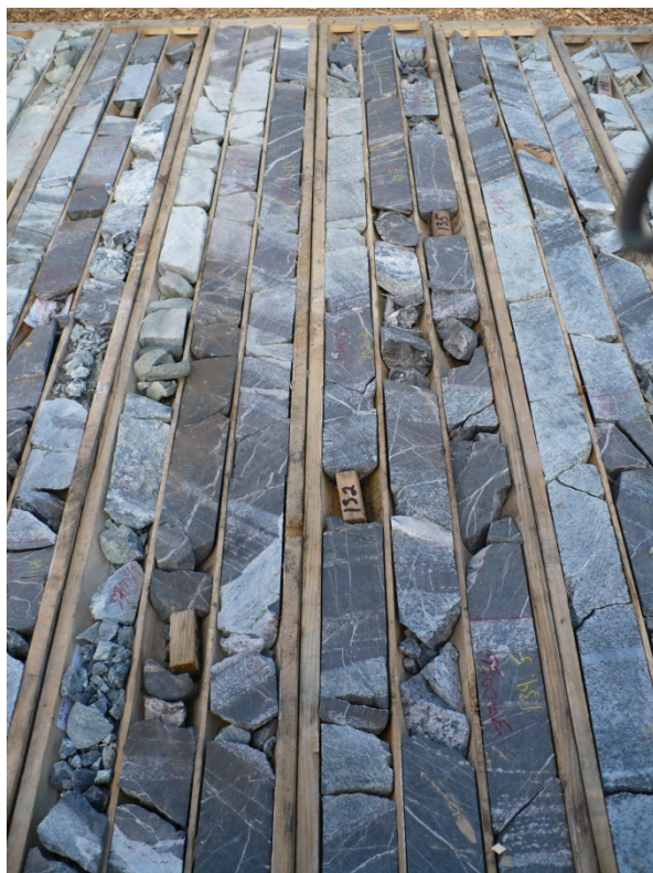
Figure 3.21. An intermittent bed of chromite shows knife sharp lower contacts and cumulus to chain chromite upper contacts with overlying olivine cumulate. Sample is from 135.8 m in DDH BT-08-10.
