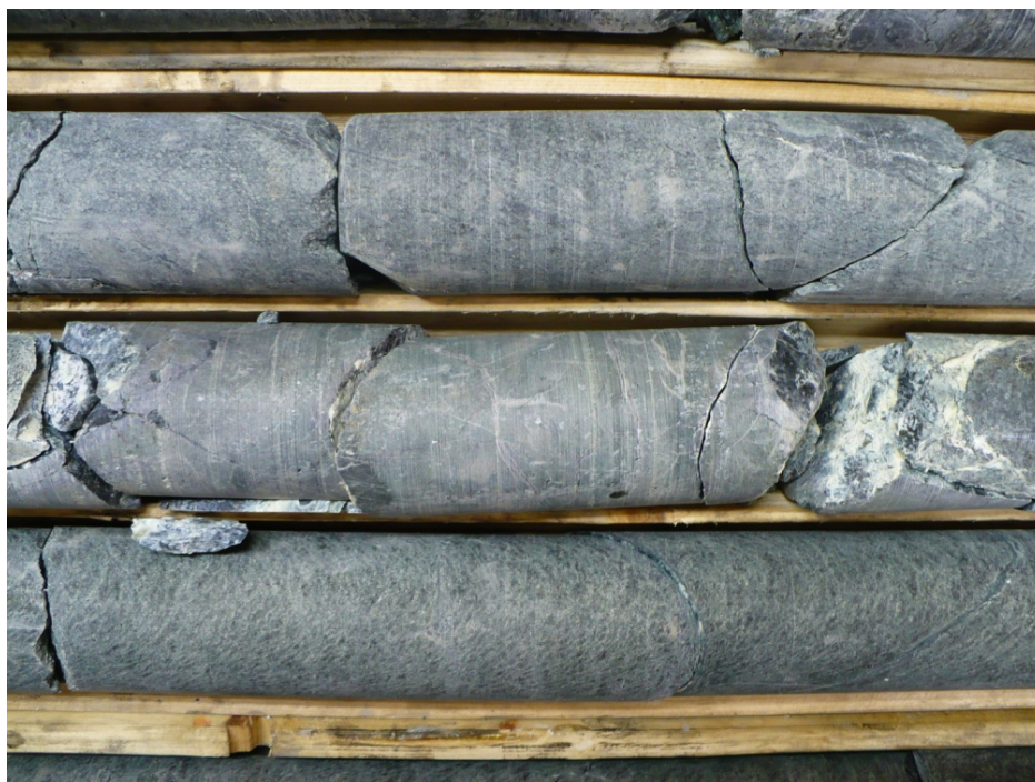
Figure 3.57. Green aphyric unit (middle core tube) is pale green and aphanitic with often the occurrence of clumps of euhedral plagioclase crystals (not shown in this sample). Sample is from 309.4 m in DDH BT-11-197. Diameter of core is 46.7 mm.
