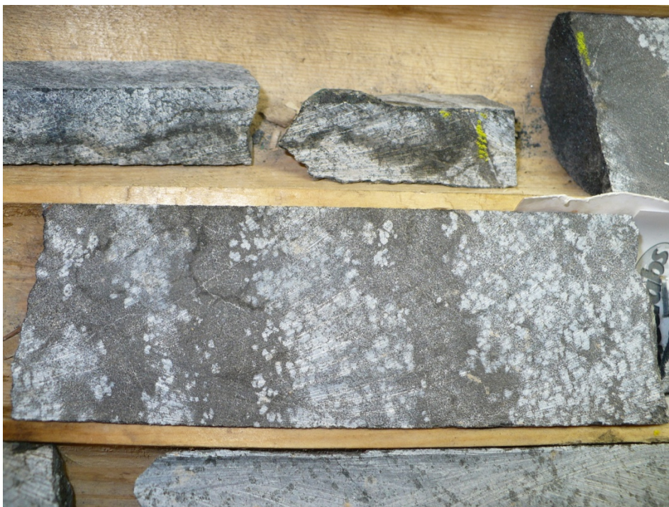
Figure 3.23. Intermittent beds of cumulus pyroxene alternating with very fine, massive cumulus chromite. Sample is from 81.80 m in DDH BT-09-17. Diameter of core is 46.7 mm.
