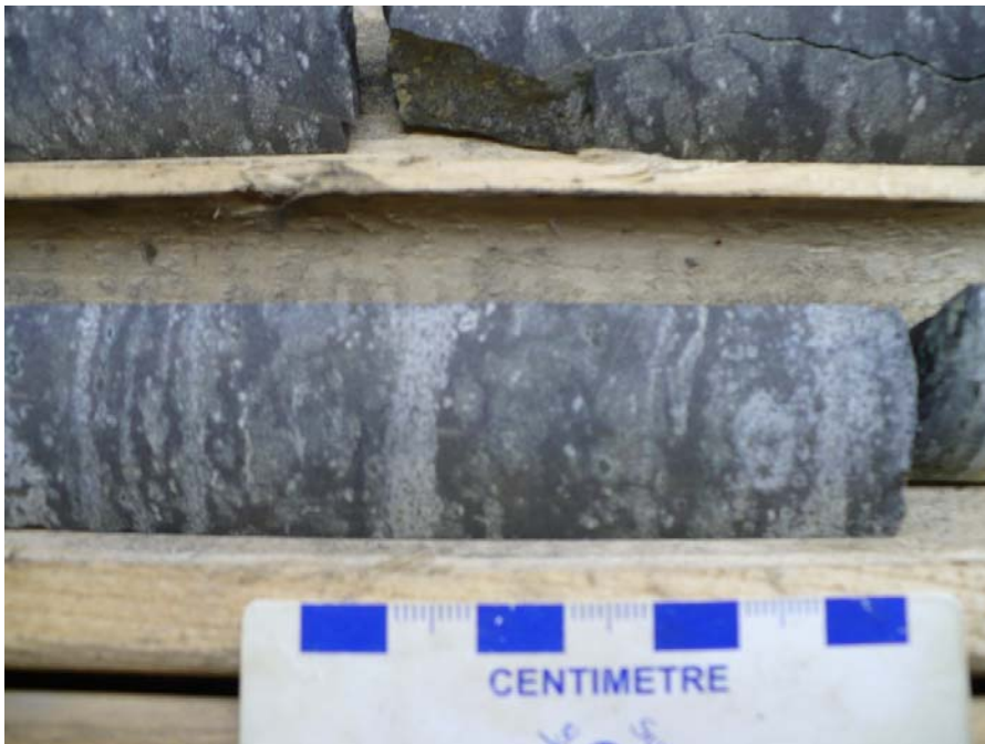
Figure 3.42. The Black Label chromitites are lower grade than Black Thor and Big Daddy chromitites. Layer 1 of Black Label is more heterogeneous and contains wavy, lensoidal and magmatic breccia textures. Sample is from 174 m in DDH BT-09-26.
