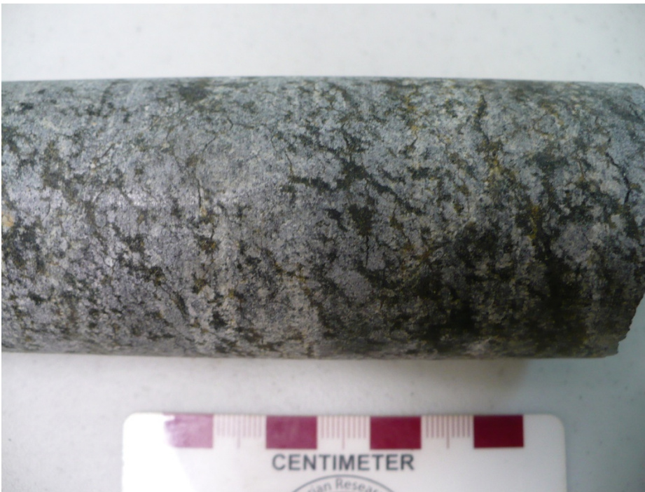
Fig. 3.51. Filter pressed olivine layers occur in another heterogeneous pyroxenite. Sample is from 173.37 m in DDH BT-09-23.
