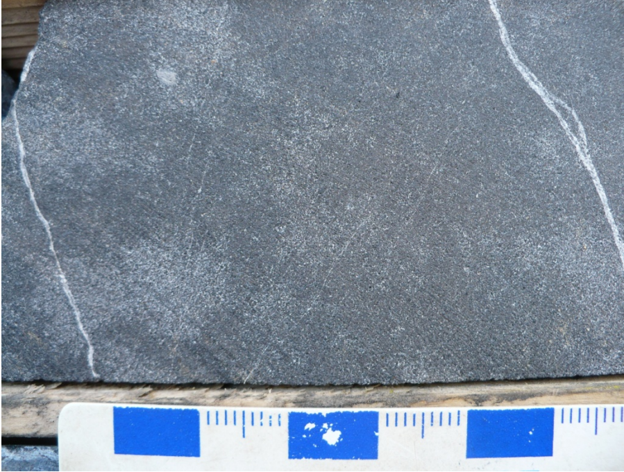
Figure 3.35. The lower Black Thor massive chromitite is the highest grade with over 90 modal % chromite. The chromitite is composed of massive granular very fine chromite with lesser intercumulus pyroxene (grey areas) content which gives the chromite a higher Cr/Fe ratio. Sample is from 160 m in DDH BT-08-10.
