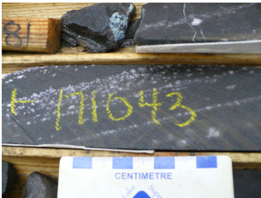
Figure 3.45. Silicate aggregate (mostly olivine) form “beaded” layers signifying magmatic layering. Sample is from 382.3 m in the Blackbird DDH NOT-08-1628.
