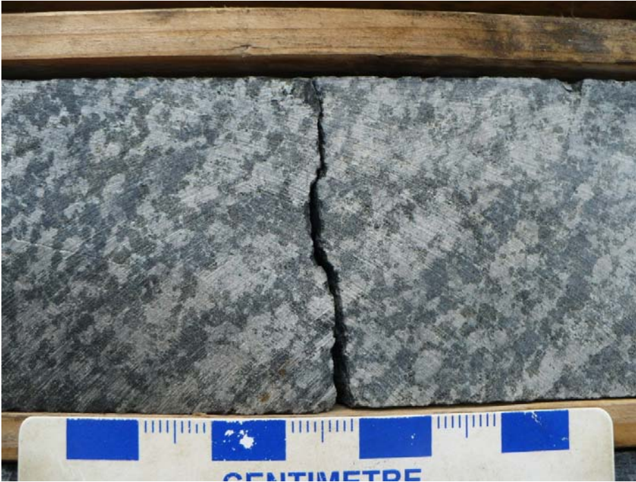
Figure 3.50. Mottled heterogeneous olivine pyroxenite contains a patchy association of 50:50 dark, fine to medium grained cumulus olivine to light grey, up to 3 mm, tremolitized, sheafy cumulus orthopyroxene. Sample is from 147.3 m in DDH FW-08-19.
