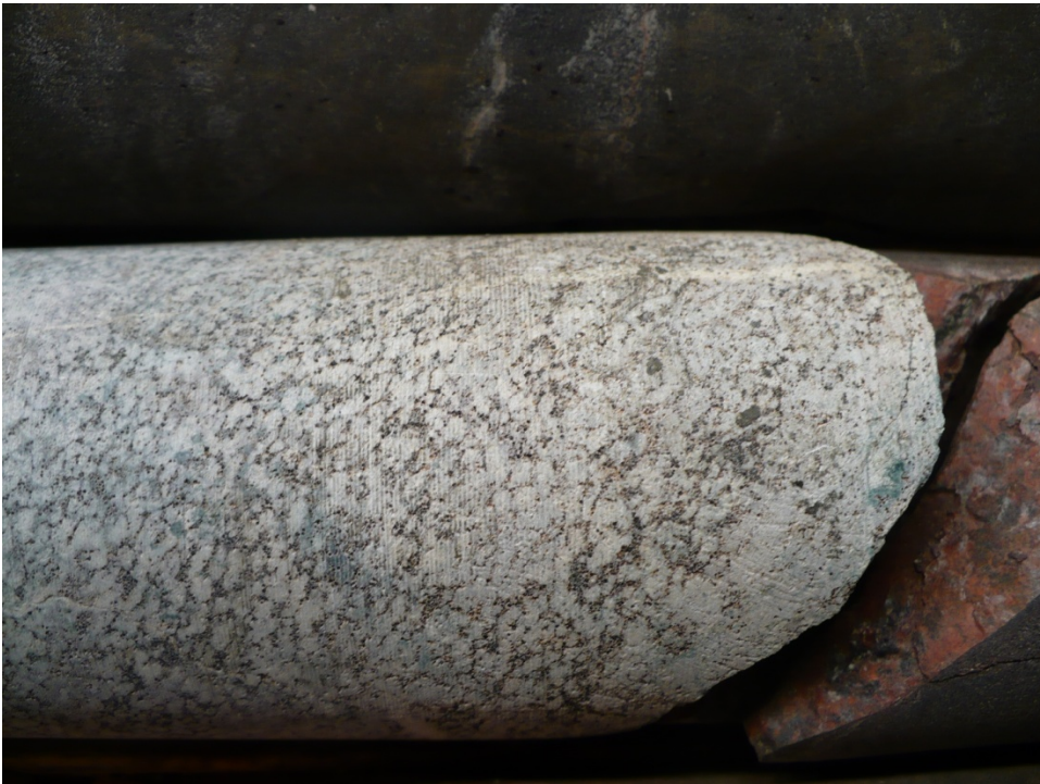
Figure 3.44. Talc altered olivines to aggregates of olivine often occur as beds in the massive chromitites. Note the red hematite alteration of the chromite on the fracture coating. Sample is from 69.75 m in DDH BT-10-133. Diameter of core is 46.7 mm.
