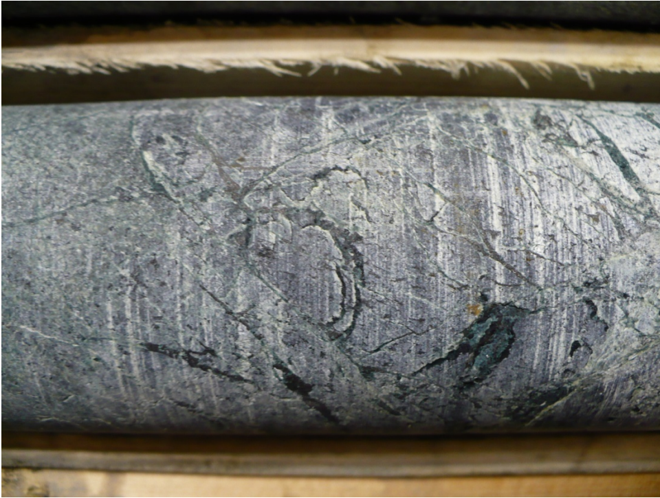
Figure 3.9. Coarse grained massive grey pyroxene at right replaces medium grained olivine. Sample is from 306.38 m in DDH BT-11-197. Diameter of core is 46.7 mm.
