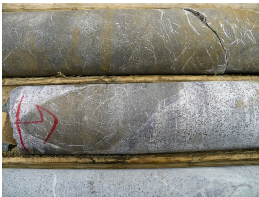
Figure 3.46. Chromitite often contains deformation fabrics proximal to pyroxenite. The brown fracturing of the chromitite lowers the Cr content. There is abundant calcite veinleting associated with the deformation. Also note the occluded silicate layering. Sample is from 474 m in DDH BT-11-200. Diameter of core is 46.7 mm.
