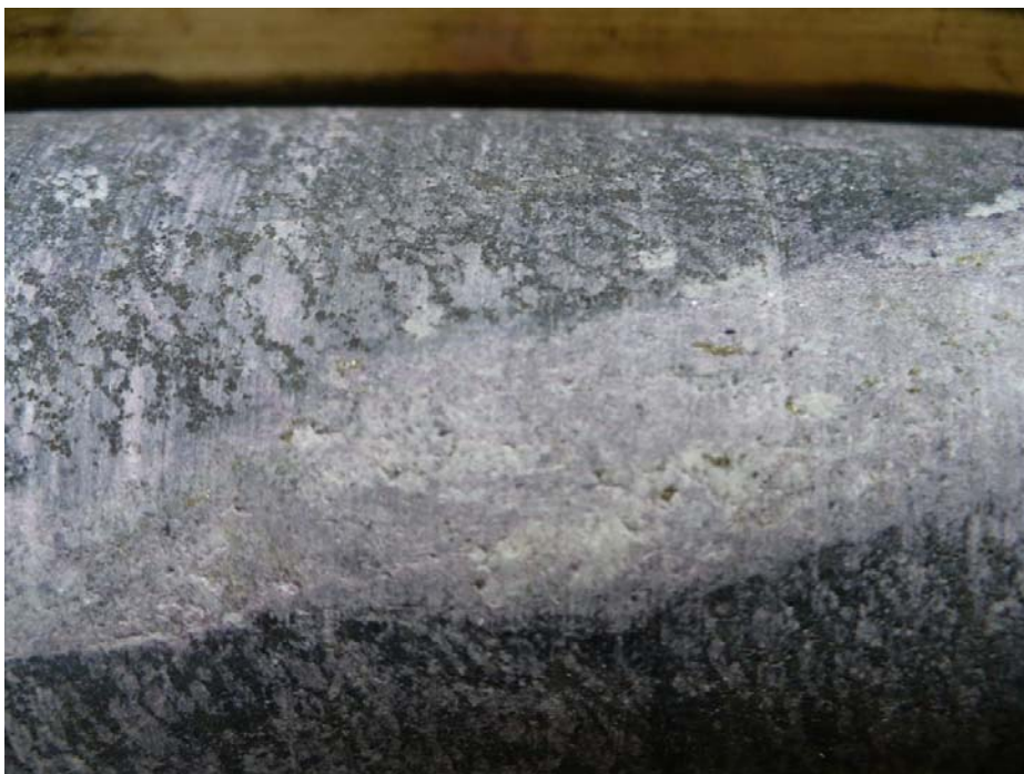
Figure 3.19. Often there is kaemmererite alteration in the chromitites. Kaemmererite is a purple, high Cr-bearing chlorite that forms due to the retrogression of pyroxene that occurs in close association with chromite. Sample is of a vein of kaemmererite that envelops coexisting dolomite and cross-cuts the chromitite. From 339.17 m in DDH FW-11-87. Diameter of core is 46.7 mm.
