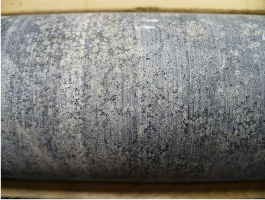
Figure 3.11. Patchy grey coarse grained pyroxene at right replaces pale grey-white talc-altered cumulus olivine. There is very fine interstitial chromite. Sample is from 381.57 m in DDH FW-11-87. Diameter of core is 46.7 mm.
