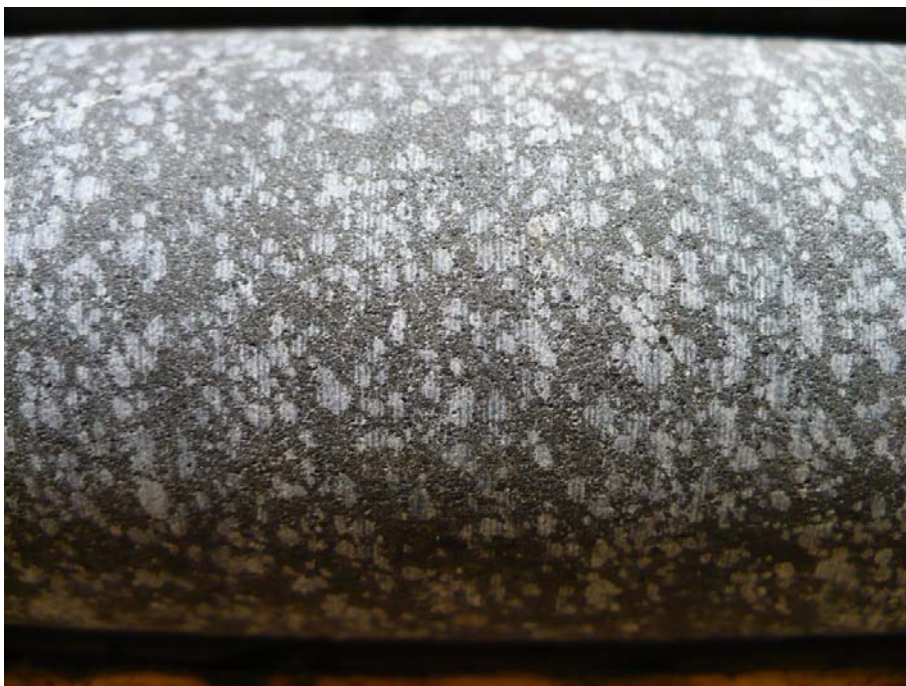
Figure 3.24. Semi massive chromite: Chromite occurs as 45 to 70 modal % interstitial very fine cumulus chromite disseminated within cumulus olivine or as dominant groundmass chromite bearing cumulus olivine. Sample is from DDH BT-11-185. Diameter of core is 46.7 mm.
