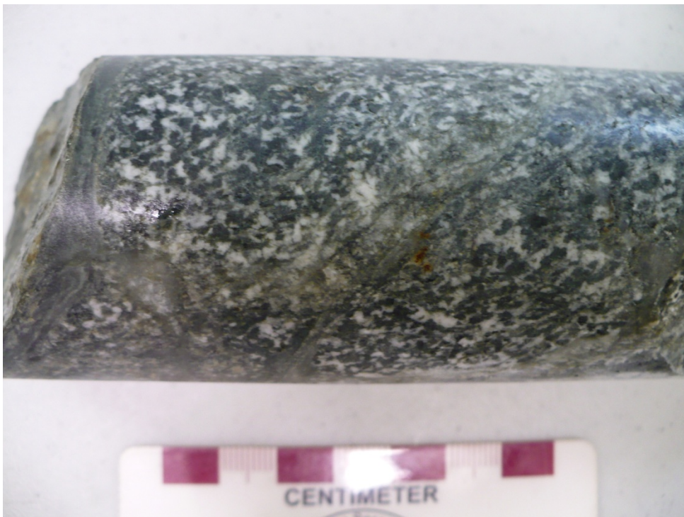
Figure 3.62. Leucogabbro is a massive light grey feldspar and quartz-phyric plagioclase-orthopyroxene cumulate. Sample is from 483.65 m in DDH BT-09-37.
