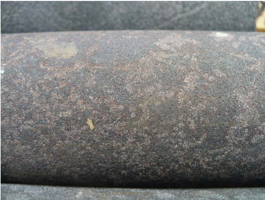
Figure 3.38. More infrequent are chicken track networks of intercumulus pyroxene in chromitite. Sample is from 94.30 m in DDH BT-10-133. Diameter of core is 46.7mm.
