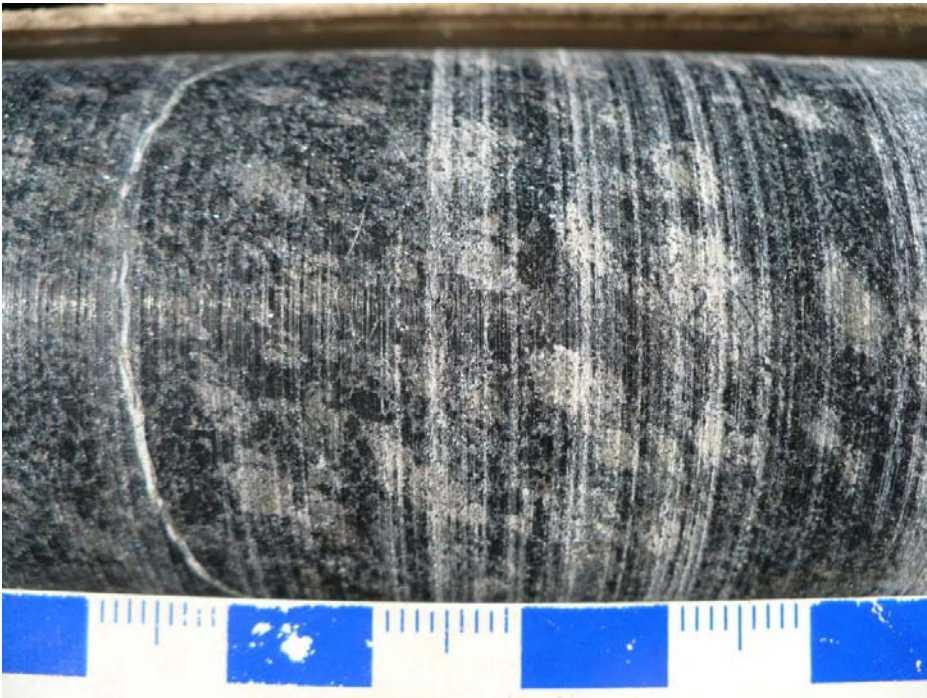
Figure 3.12. Harzburgite containing 35 modal % 1 cm oval to rounded tremolitized oikocrysts of pyroxene in serpentinized fine grained dark cumulus olivine groundmass. Sample is from 143.6 m in DDH BT-09-31.
