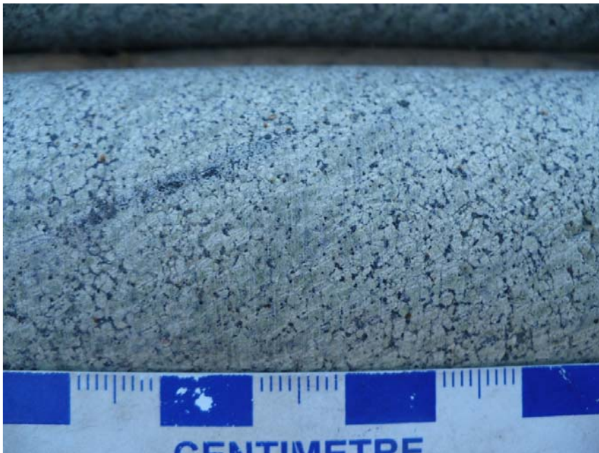
Figure 3.6. Dunite is composed of light green fine grained round cumulus serpentinized olivine with interstitial chromite. Sample is from 33.48 m in DDH BT-08-08.
