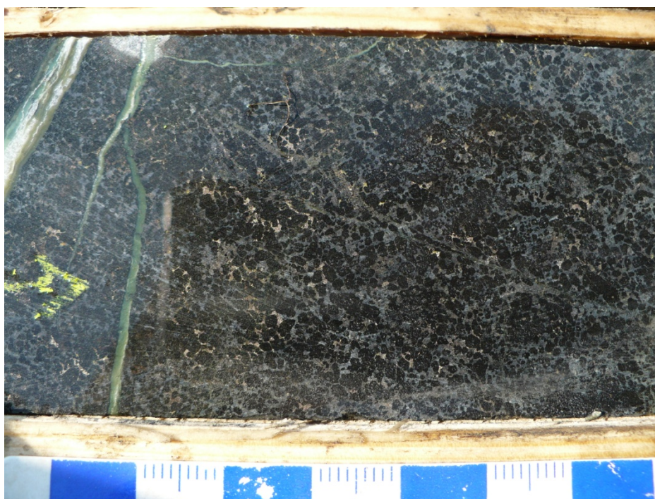
Figure 3.49. Fine interstitial po-pn-cpy sulphides in magmatic breccia. Sample is from 244.68 m in DDH BT-09-29.
