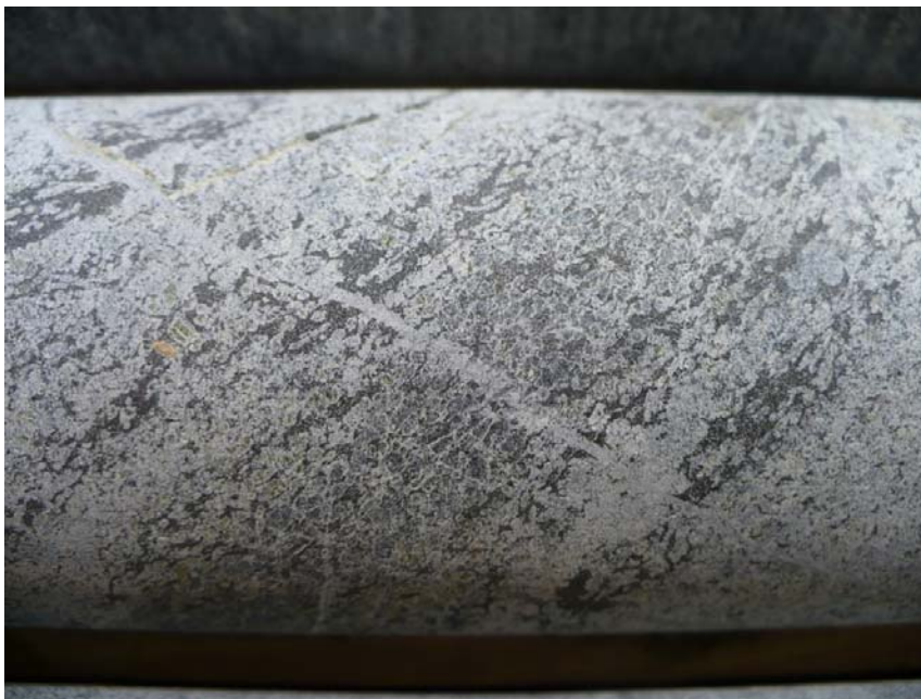
Figure 3.55. Pyroxenite occasionally contains disseminated chromite in the form of wispy interstitial chromite and bands that are finer grained than chromite in dunite. Sample is from 102.7 m in DDH BT-09-17. Diameter of core is 46.7 mm.
