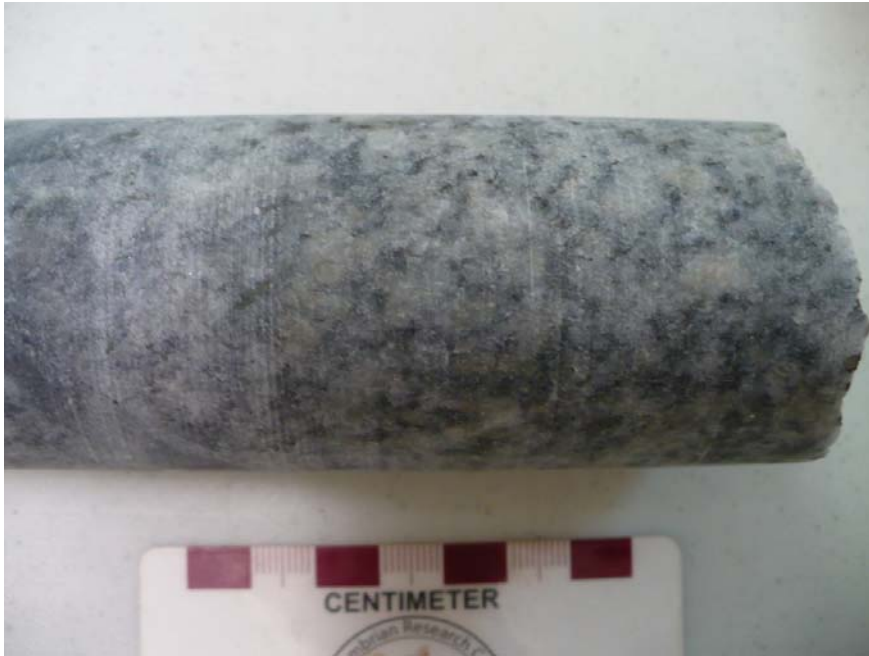
Figure 3.5. Granodiorite is basement to the Ring of Fire Intrusion. Sample is from 148.33 m in DDH BT-09-62.
