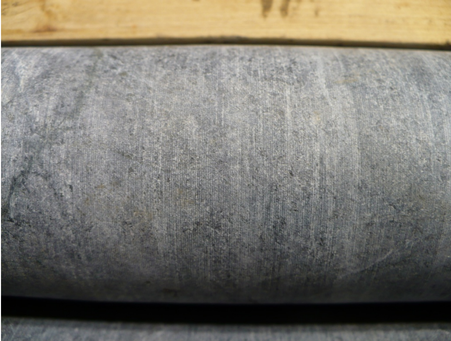
Figure 3.52. Pyroxenites are light grey medium to coarse grained massive units composed of sheafy to tabular, cumulus pyroxene. Sample is from 35 m in DDH BT-10-133. Diameter of core is 46.7 mm.
