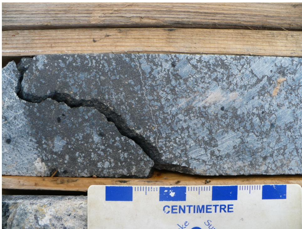
Figure 3.21. An intermittent bed of chromite shows knife sharp lower contacts and cumulus to chain chromite upper contacts with overlying olivine cumulate. Sample is from 135.8 m in DDH BT-08-10.
