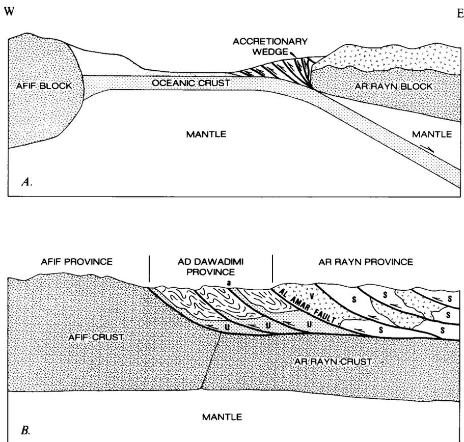
FIG. 5. Generalized geological cross section of the Halaban-Al Amar region. (A) At 680 Ma, shortly before plate collision, and (B) at 640 Ma, the end of collision. Unit symbols: a, Abt schist; u, ophiolitic complexes of the Urd group; v, volcanic and sedimentary rocks of the Al Amar group; s, syntectonic plutonic rocks.
