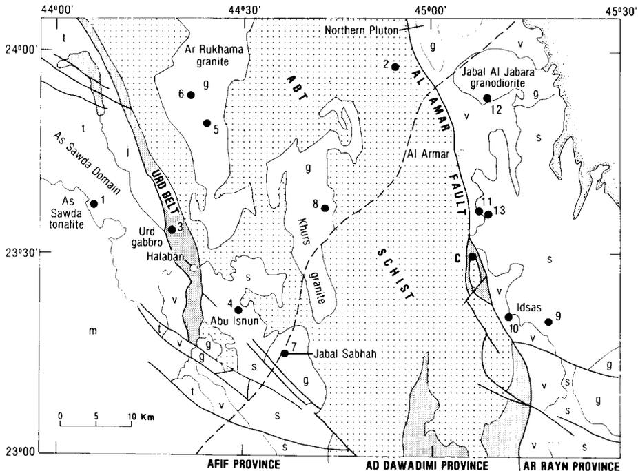
FIG. 2. Simplified geological map of a part of the Halaban-Al Amar region showing sample localities (locality numbers from Table 1). C indicates trondhjemite with 2000 Ma zircons of Calvez *et al.* (1983). The deep seismic line of Healy *et al.* (1982) is shown by the dashed line.
